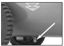
Figure 5. Drain valve location.
